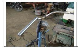
Bike Use Handle for accelerator with brake Lever.
