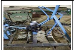
Remove Pedal And use 24 V. 250 watt D.C. Motor
